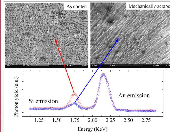
Solid AuSi eutectic surface is enriched in Si; mechanically scraped surface reveals alloy close to eutectic composition (above)
