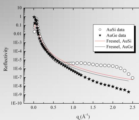
Specular x-ray reflectivity shows that AuSi surface reflects noticeably stronger signal than the AuGe surface.
