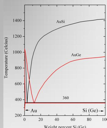
Melting point of AuSi and AuGe eutectic is about 360°C; this temperature is significantly lower than melting point of Au (1064°C), Si (1410°C) or Ge (937°C)
