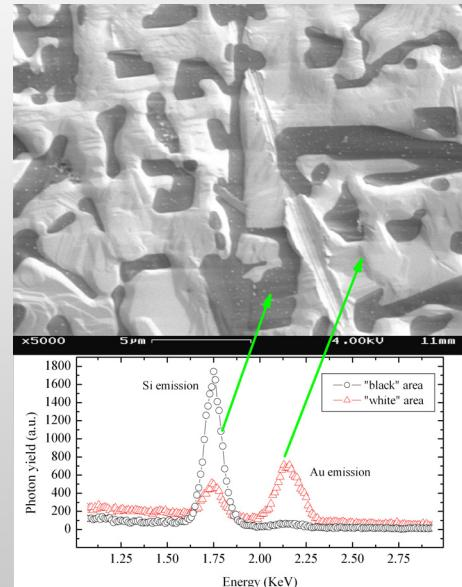
The solid surface consists of patches of Si rich alloy and almost pure Si (right)
