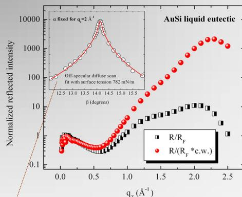
Off-specular diffuse scattering (the inset) proves liquid character of the surface.
