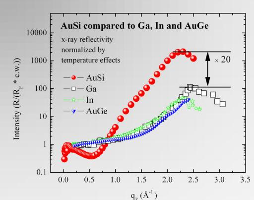
Maximum amplitude of normalized surface form factor squared is ~20 times larger than measured for any other pure metal or alloy.
