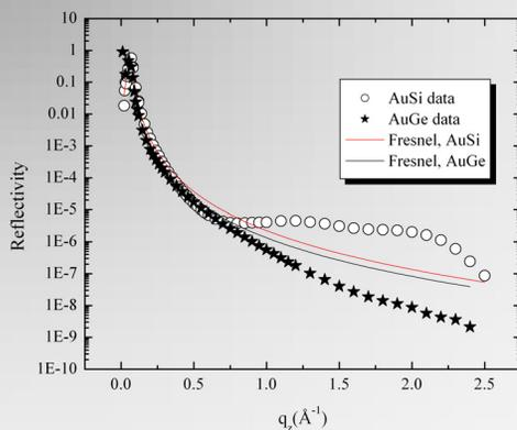
Specular x-ray reflectivity shows that AuSi surface reflects noticeably stronger signal than the AuGe surface.
