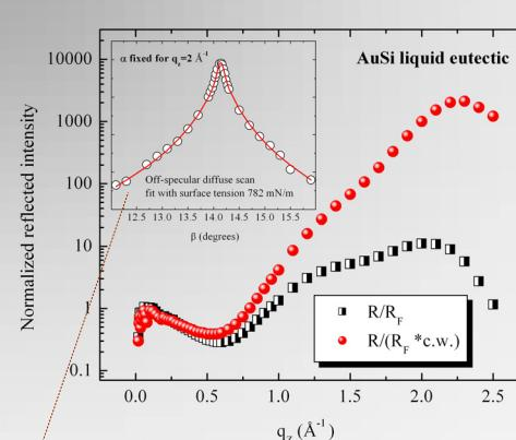
Off-specular diffuse scattering (the inset) proves liquid character of the surface.
