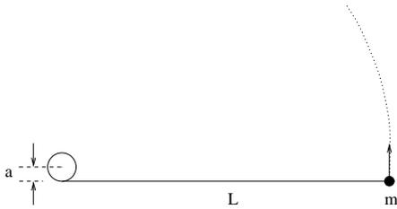
At a given time, a vertical pole (of radius  $a$ , with  $a \ll L$ ) is fixed onto the table next to the center of the circle, as shown. The spring winds around, and the mass eventually hits the pole. Assume that the pole is sticky, so that any part of the spring touching the pole does not slip. How long does it take for the mass to hit the pole?
