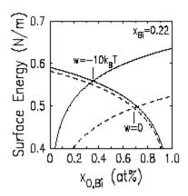
Surface free energy condition equating surface tension and entropic terms for In and Bi as functions of concentration.
