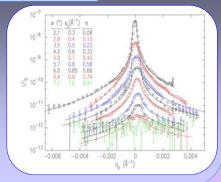
Surface Structure Factor (Squared): Fresnelnormalized reflectivity with thermal (capillary) effects taken out, for Ga, K, water
